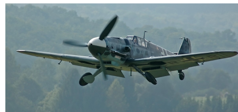
A Bf 109G-6 taking off. The bulges of the MG 131s on the cowling and of the enlarged tyres on the upper wings are clearly seen in this machine, earning the G-6 the name “The Bump” by its pilots.
