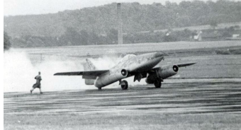
A Me 262 prototype in 1943. Note the tail wheel instead of the nose wheel of the production aircraft.
