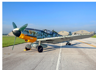
A Bf 109G-10 with streamlined cowling bulges. Courtesy of the National Museum of the United States Air Force.
