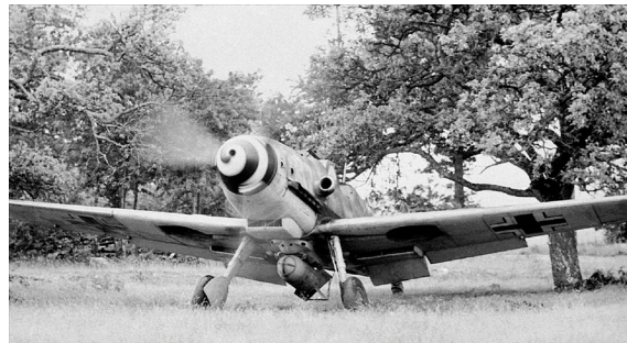
A Bf 109G loaded with a 250 kg bomb warms up its engine before a strike mission.
