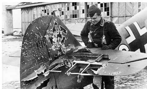
A ground crewman inspects the damaged tail of a Bf 109 after a combat sortie.
